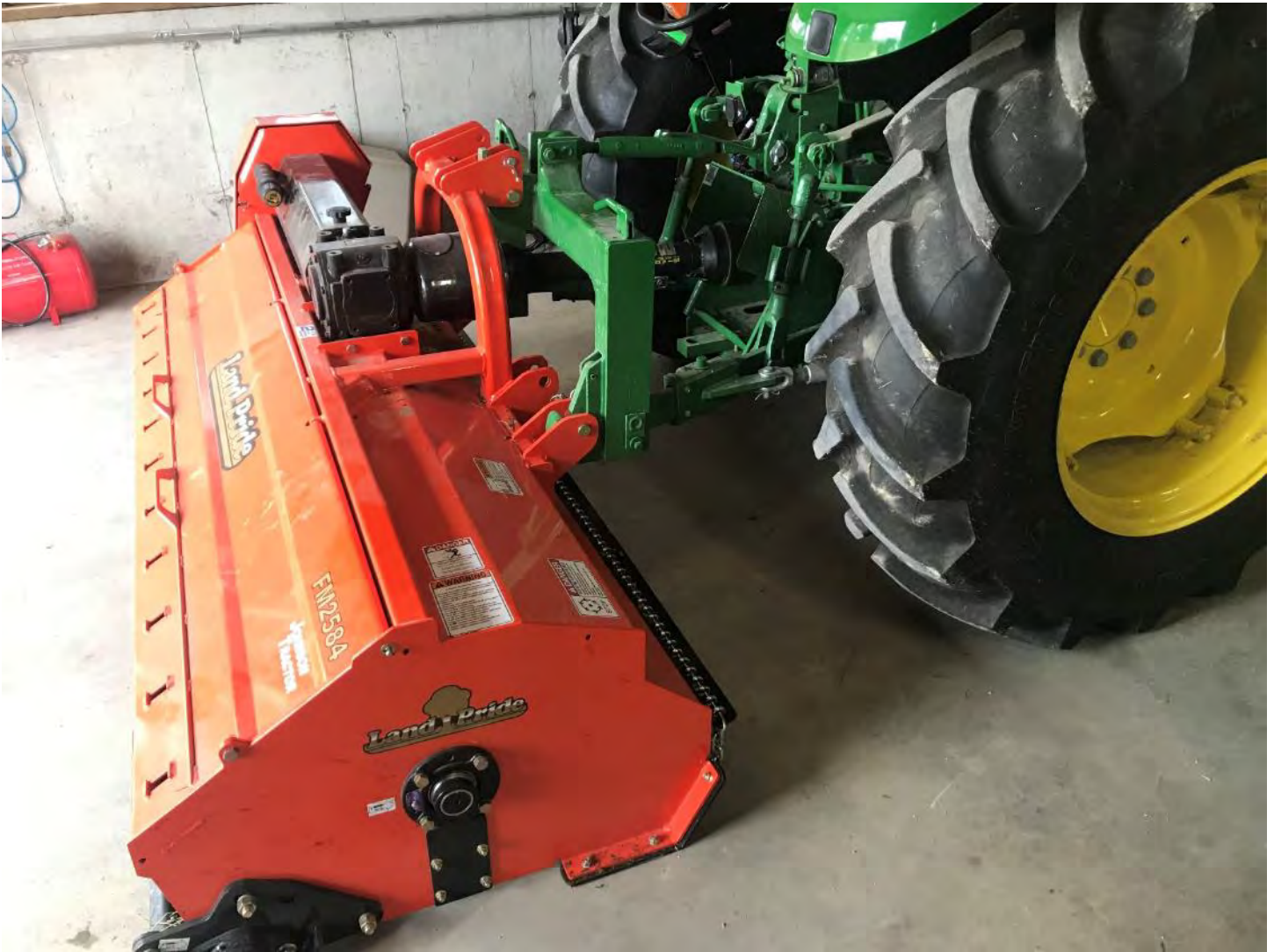
This is a flail mower, rather than a rotary mower. This is a new tool for us. It mows fire breaks very short and shreds the material.
